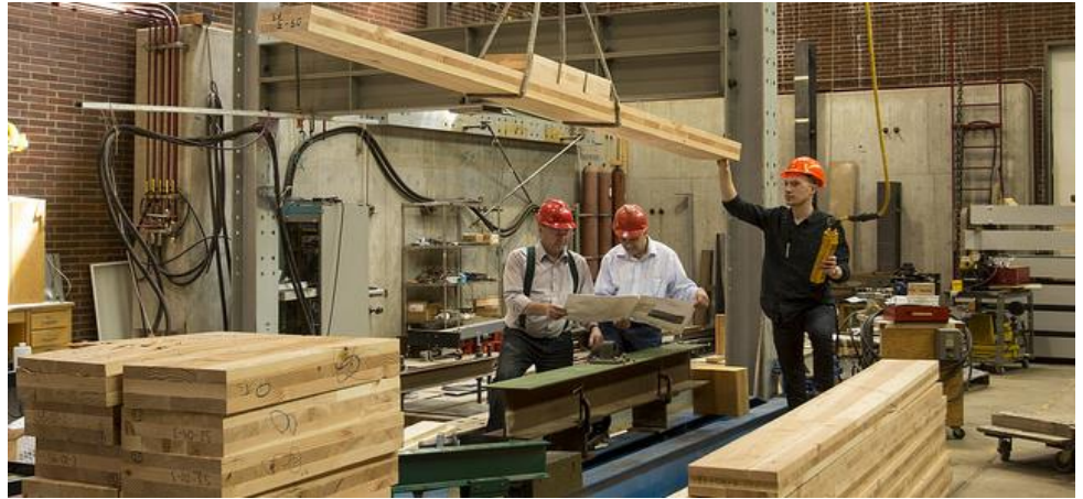
Cross-Laminated Timber (CLT) is a sustainable engineered wood product developed in the OSU College of Forestry and manufactured by several Oregon timber companies.
