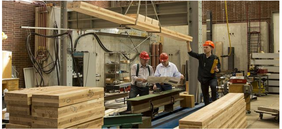
Cross-Laminated Timber (CLT) is a sustainable engineered wood product developed in the OSU College of Forestry and manufactured by several Oregon timber companies.
